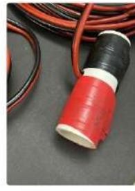
ROV Power Connection
